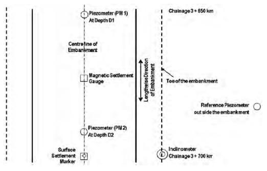
Fig. 6.12 Typical Plan for Instrument Installation in Embankment over Soft Soil
