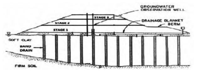
Fig. 5.1 Typical Cross Section of PVD Installation for Embankments
