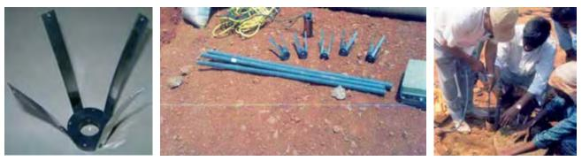
Fig. 6.6 Magnetic Spider, PVC Access Tubes and Installation of Magnetic Settlement Gauge
