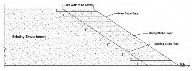
Fig. 8 (a) Widening of Embankment by cutting Benches and Filling
