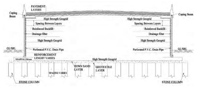
Fig. 5.7 Pile supported Basal Reinforced Embankment
