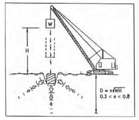
Fig. 5.3 Systematic Arrangement of Dynamic Compaction
