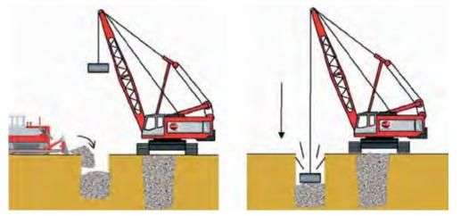
Fig 5.5 Construction Sequence Dynamic Replacement
