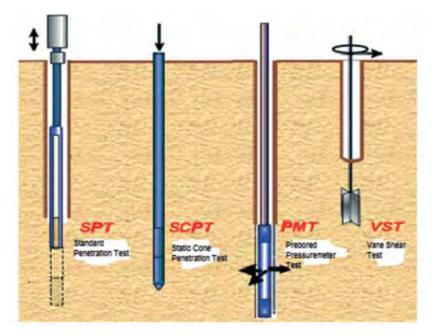
Fig. 2.2 Schematic Representation of various In-situ Tests
