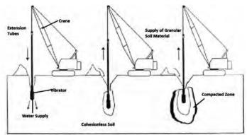
Fig. 5.4 Vibro Compaction Process
