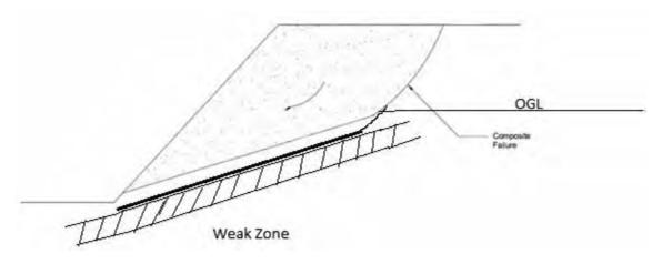
Fig. 3.1.b Composite Failures along non Circular Surface
