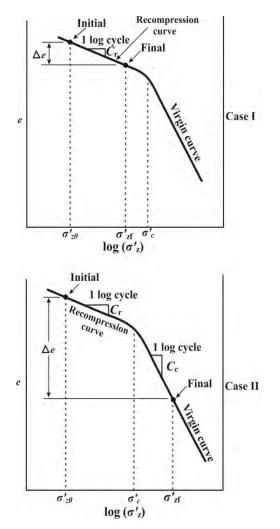
Fig. 4.1 Consolidation of Over-consolidated Soil
