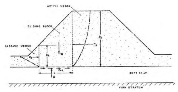
Fig. 3.8 Sliding Block Analysis
