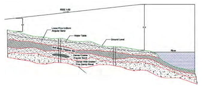
Fig. 2.3 Longitudinal Profile of the Subsoil
