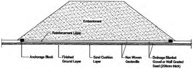
Fig. 5.6 Basal Reinforced Embankments (for more details, refer IRC:113)
