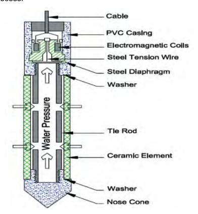
Fig. 6.4 Vibrating Wire Piezometer
