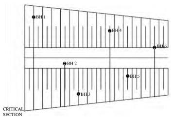
Fig. 2.1 General Boring Layout for High Embankments
