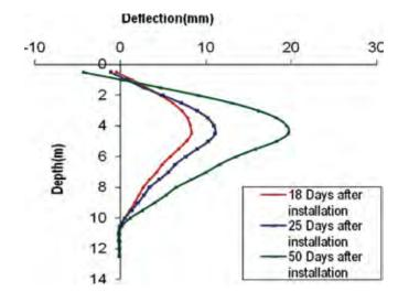
Fig. 6.10 Typical Inclinometer Output
