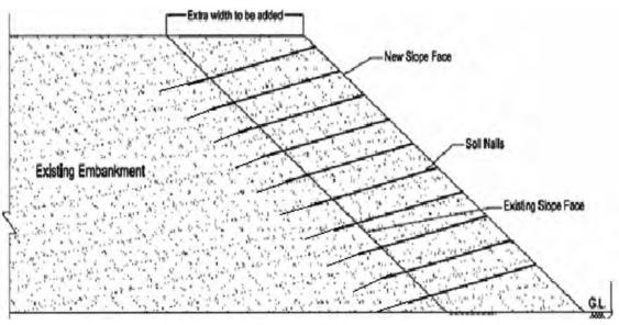
Fig. 8 (b) Widening of Embankment using Soil Nailing
