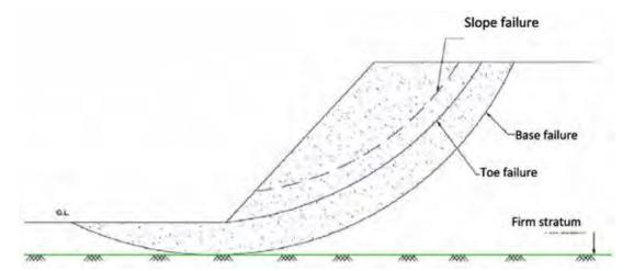
Fig. 3.1.a Rotational Failure Along Circular Surface
