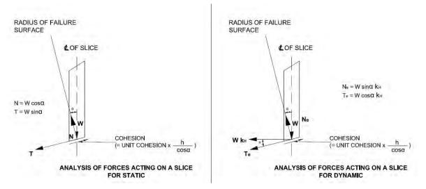
Fig. 3.9 Analyses of Earthquake Induced Forces (Circular Arc Method – Method of Slices)
