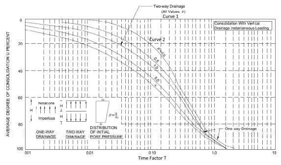
Fig. 4.2 Time Factors for Consolidation Analysis
