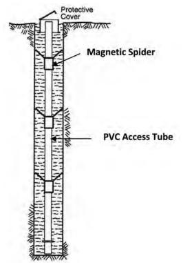
Fig. 6.7 Parts of Magnetic Settlement Gauge
